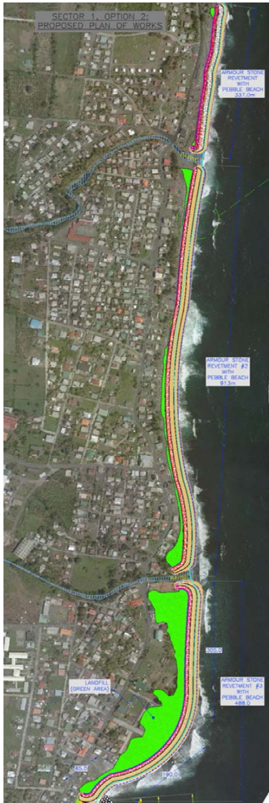
Figure 6.3: Preferred Option for Sector 1 – Protective Armour Stone Revetment/Buffer Zone & Nourishment (Source: Task 2 Report)
